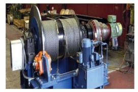
VOLDRUM Tugger Haulage Products and after engineered designed by Voltas to haul coal tubs at faces. It is one of the oldest product in its category operating across various underground coal mines in India.
