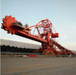
Bulk Material Handling Products Voltas also brings to its stable a host of bulk material handling products used in handling of Ore or Coal bulk. The product ranges under this stable includes apron feeder,feeder breaker,sizer and Stacker Reclaimer.
